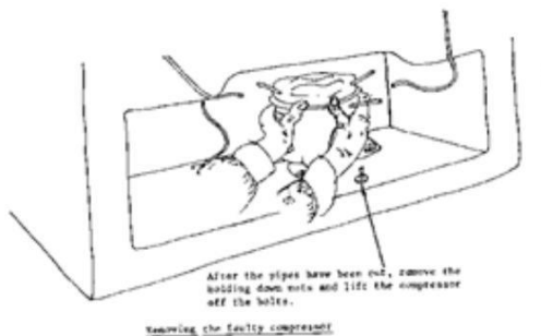
Figure 50. Remove faulty compressor
