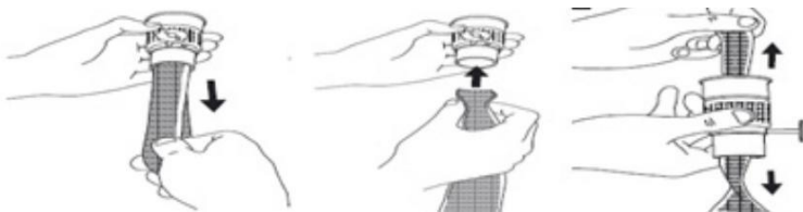
Figure 21. Inserting the new wick
