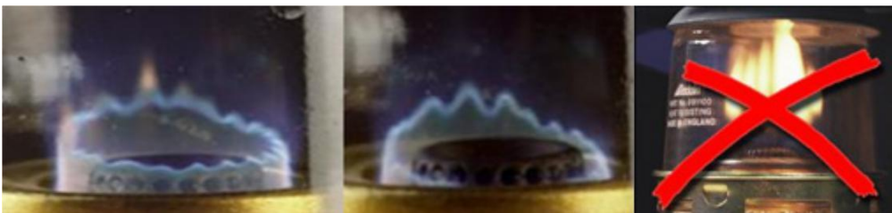
Figure 19. Adjusting the minimum and maximum setting of flame Figure 20. Wrong yellow flame
