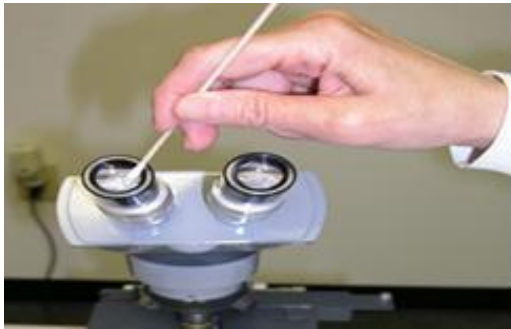
Figure 2 cleaning an eye piece
