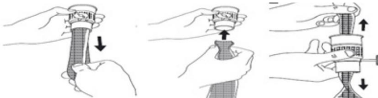
Figure 21. Inserting the new wick
