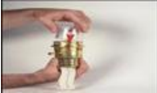
Figure 11. Reassemble the burner gallery
