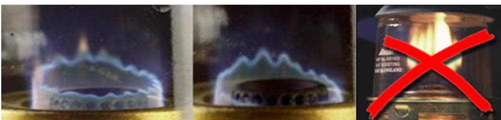
Figure 19. Adjusting the minimum and maximum setting of flame Figure 20. Wrong yellow flame
