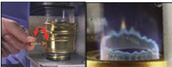
Figure 18. Adjusting the burner for proper flame
